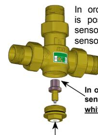
In order to modify the valve setting, it is possible to replace the thermostatic sensor: unscrew the plug, remove the sensor by hand and position the new one.
